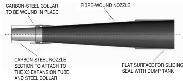
Figure 5: Sketch of the X3 steady expansion nozzle [2]
