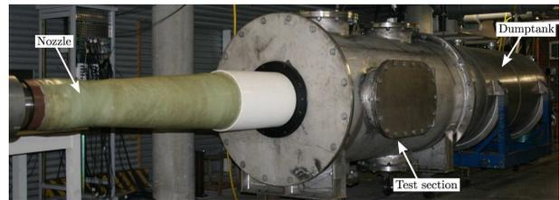
Figure 6: X3 nozzle, test section and dump tank [5]
