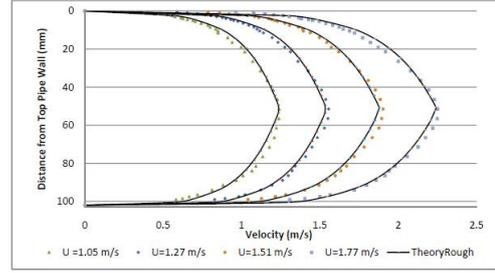
Figure 9: Comparison between measured and modified theoretical velocity profiles in the fouled test section with  $\kappa$  and  $B$  varied for each test case
