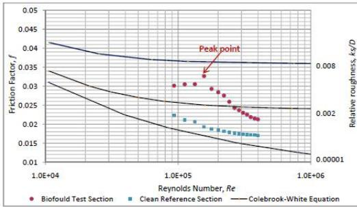
Figure 3: Moody diagram showing experimental and predicted values of friction factor
