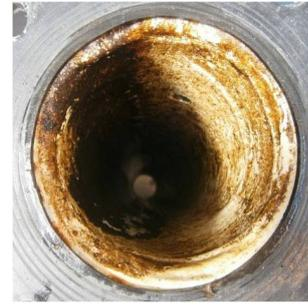
Figure 5: Photograph of flow conditioned biofouling inside the test section after testing
