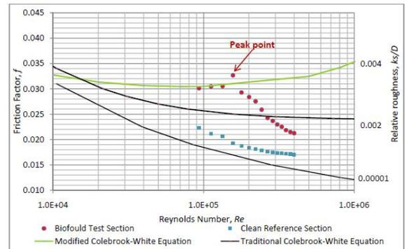
Figure 6: Moody diagram showing experimental, predicted (original and modified) values of friction factor
