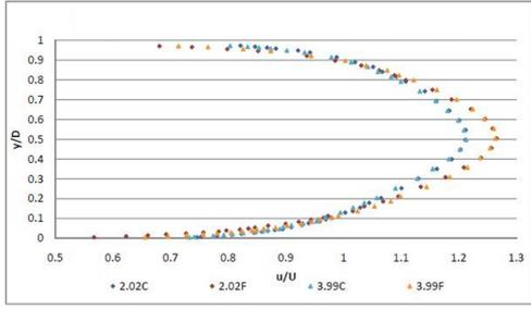
Figure 7: Non-dimensional velocity profiles of the test section with biofouling for clean (C) and fouled (F) pipes
