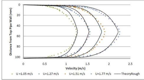
Figure 8: Comparison between measured and theoretical velocity profiles in the fouled test section with  $\kappa = 0.4$  and  $B = 8.48$
