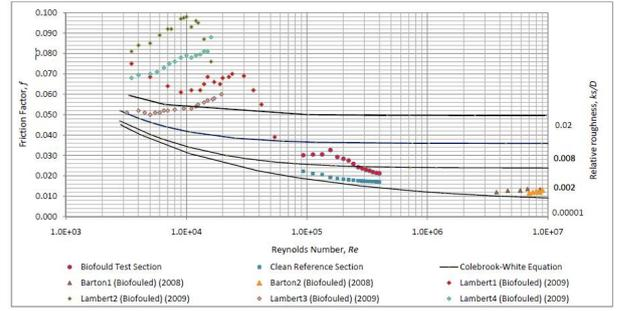
Figure 4: Moody diagram showing experimental predicted values of friction factor for a range of experimental programs
