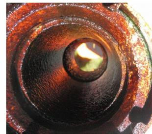
Figure 2: Photograph of flow conditioned biofouling inside the test section before testing
