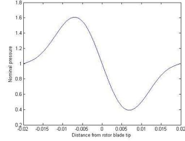
Figure 5 Analytical pressure distribution across blade sector span
