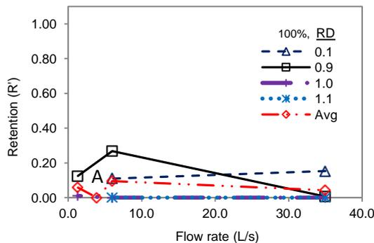
Figure 4. Normalised capture/retention profiles ( $R'$ ) for continuously fed variable density spheres ( $RD = 0.1, 0.9, 1.0$  and  $1.1$ ). The channel inlet configured GPT experiment is with fully blocked screens tested under varying flow rates (See table 1). A (See left of figure) denotes poor capture/retention performance which may be attribute to large negative velocities denoted by B in figure 3.
