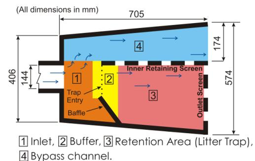
Figure 2. Plan view of gross pollutant trap—LitterBank—with labelled sections.
