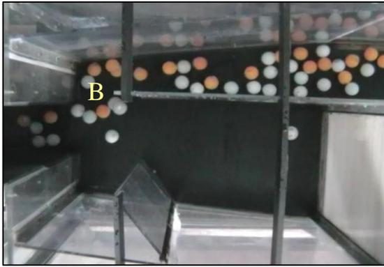
Figure 3. Left, experiments with fully blocked screen show the neutrally buoyant spheres ( $RD = 1.0$ ) escaping the GPT via the bypass (See data point A in figure 4 at  $1.3$  L/s on the abscissa—see table 1). B (See left of figure) denotes the existence of large negative horizontal velocities (right to left).
