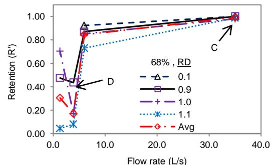
Figure 6. Normalised capture/retention profiles ( $R'$ ) for continuously fed variable density spheres ( $RD = 0.1, 0.9, 1.0$  and  $1.1$ ). The channel-inlet-configured GPT experiment is with 68% blocked screens tested under varying flow rates (table 1). See snapshots of capture/retention performances in figures 5 and 7 for C and D, respectively.
