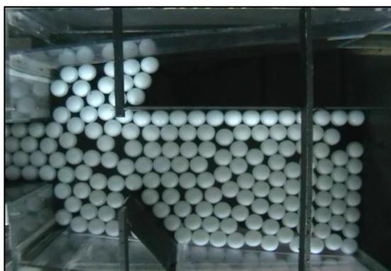
Figure 7. Single layer deposition pattern for the GPT with 68% blocked screen capture/retention of the lightest pollutants (RD = 0.9) at a low (3.9 L/s) flow rate (See D, figure 6).
