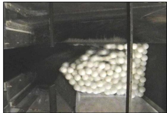
Figure 5. Deposition pattern for the GPT with 68% blocked screen shows total (100%) capture/retention of the lightest pollutants ( $RD = 0.1$ ) at a high ( $35$  L/s—Table 1) flow rate (See C, figure 6).
