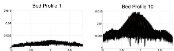
Figure 3. Initial and final deposit profile from the distal end of basin. Note the symmetrical nature of the latter deposit (dimensions in metres).
