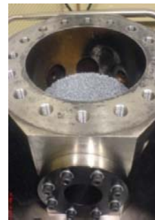
Figure 3: Top view of porous medium inside CVC.
