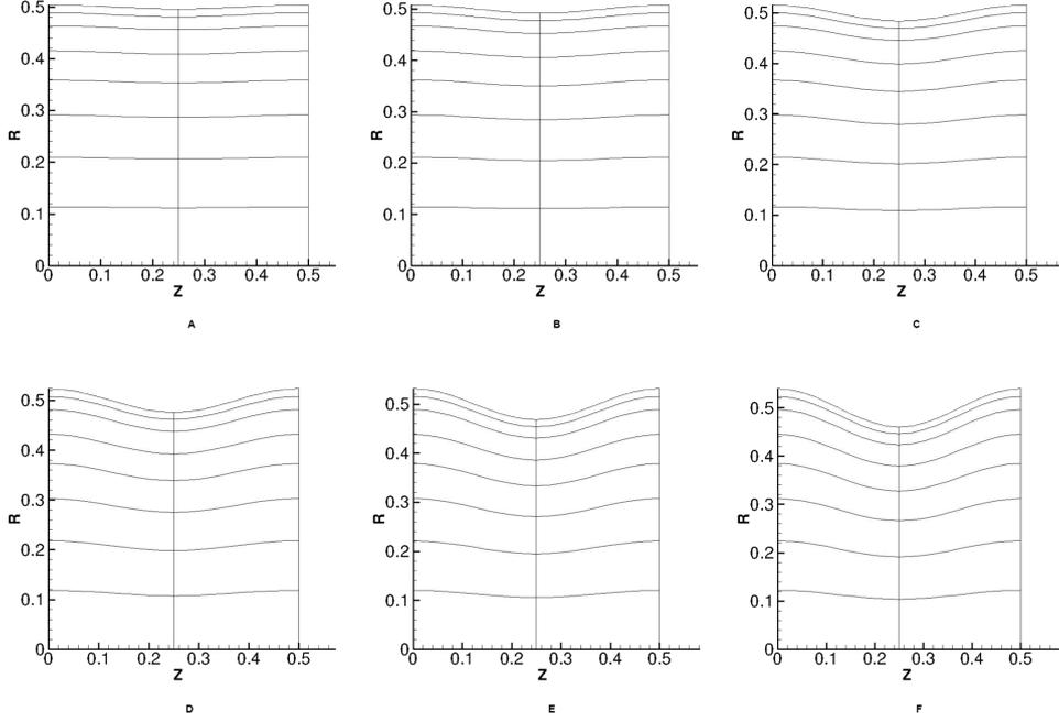
Figure 1: Spectral element meshes used. Non-dimensional corrugation amplitudes are (a)  $a=0.015904$  (b)  $a=0.031808$ , (c)  $a=0.063612$ , (d)  $a=0.095420$ , (e)  $a=0.127228$ , (f)  $a=0.159032$
