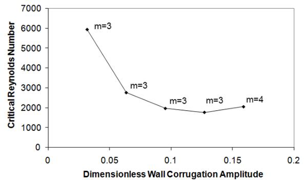
Figure 5: Critical Reynolds number against dimensionless wall corrugation amplitude for non-axisymmetric disturbances
