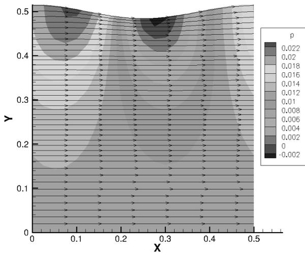
Figure 2: Laminar base flow attached to the wall for the entire computational domain. Dimensionless wall corrugation amplitude is 0.063612, bulk flow Reynolds number is 1790, contours of pressure shown with streamlines.
