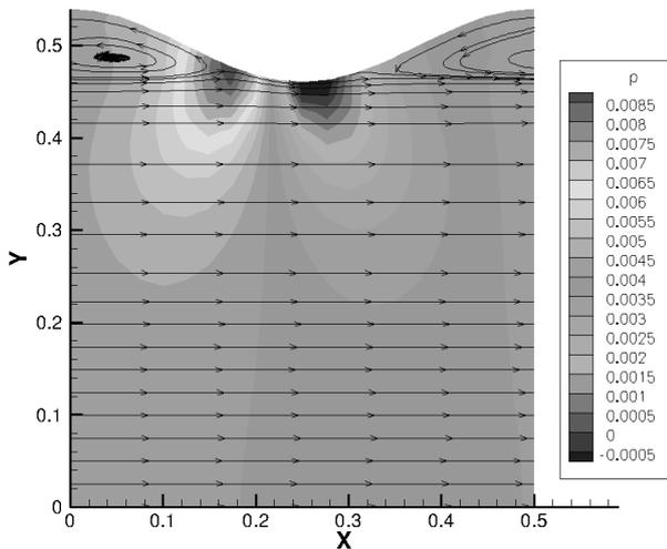
Figure 3: Base flow detached from the wall with a recirculation zone between corrugations, dimensionless wall corrugation amplitude is 0.159032, bulk flow Reynolds number is 7990, contours of pressure shown with streamlines.
