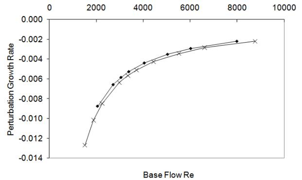
Figure 4: Growth rate of axisymmetric perturbations against bulk flow Reynolds number for dimensionless corrugation amplitudes  $a=0.159032$  (dots) and  $a=0.127228$  (crosses).
