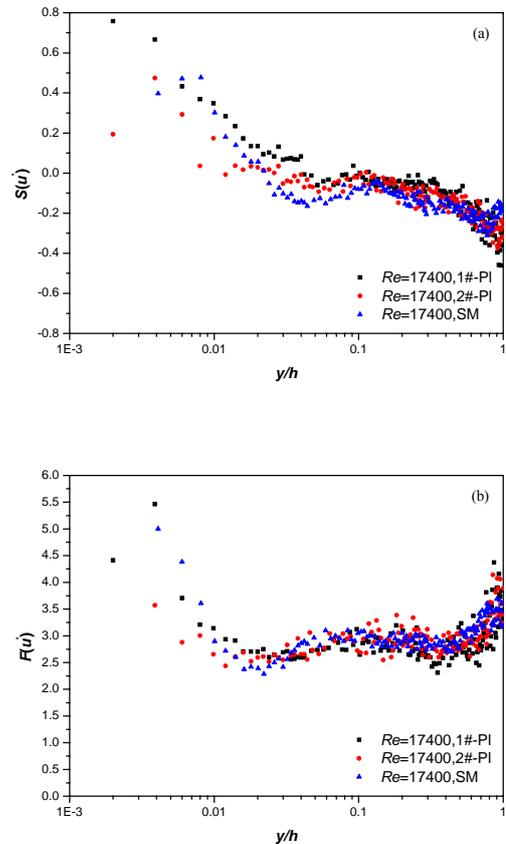
Figure 5. Higher-order moments of streamwise component over the half channel height for different rough surfaces. (a) Skewness factor and (b) Flatness factor.
