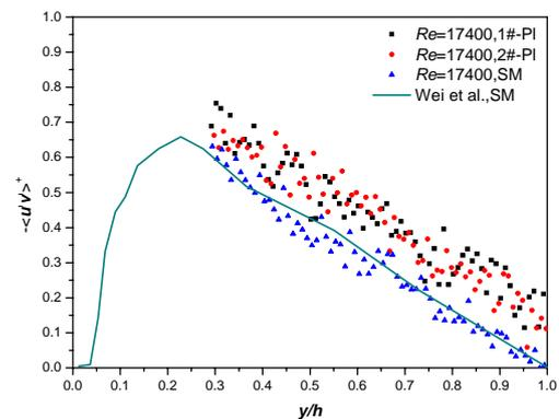
Figure 6. Reynolds shear stress distributions in the outer region for different rough surfaces. Symbols are for present experiments; Solid line is for LDV measurements of Wei et al. [14].
