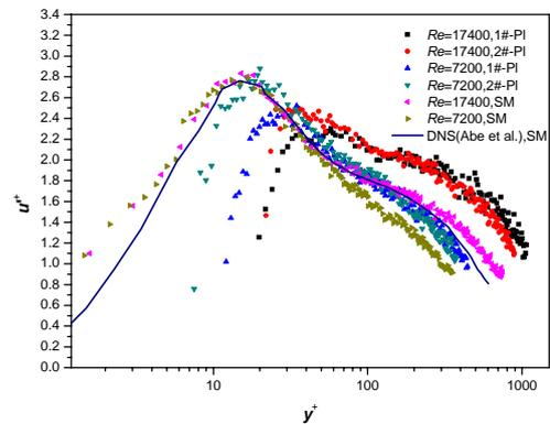
Figure 3. Streamwise turbulence intensity distributions normalized by inner variables for different rough surfaces. Symbols are for present experiments; Solid line for DNS of Abe et al. [1].
