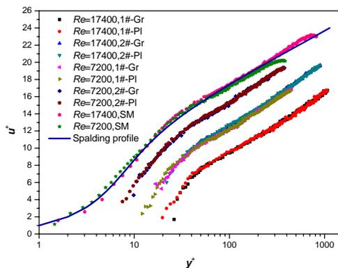
Figure 2. Streamwise mean velocity distributions normalized by inner variables for different rough surfaces.
