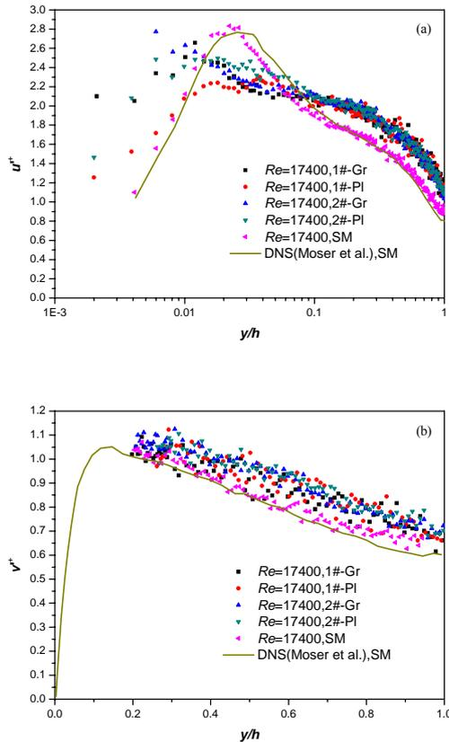
Figure 4. Turbulence intensity distributions normalized in global coordinates. (a) Streamwise; (b) Wall-normal. Symbols are for present experiments; Solid line is for DNS of Moser et al. [7].
