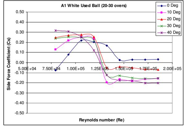
Figure 10.  $C_S$  variation with Re for used ball (20-30 overs)
