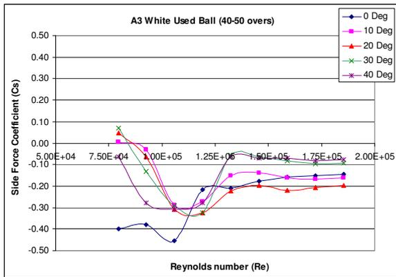
Figure 11.  $C_s$  variation with Re for used ball (40-50 overs)
