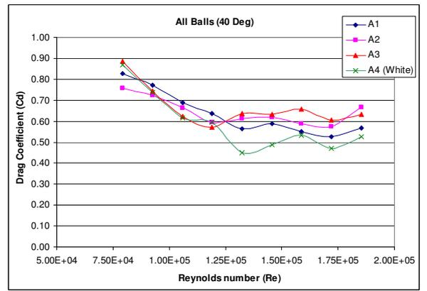
Figure 8.  $C_D$  variation with Re for all balls at  $40^\circ$  seam angle
