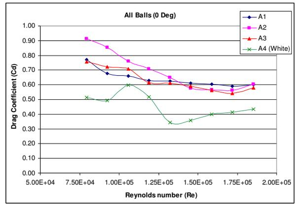
Figure 7.  $C_D$  variation with Re for all balls at  $0^\circ$  seam angle
