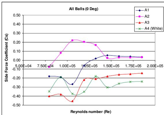
Figure 13.  $C_s$  variation with Re for all balls at 0° seam angle
