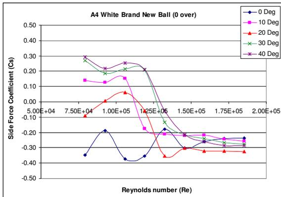
Figure 12.  $C_s$  variation with Re for a new ball (0 over)
