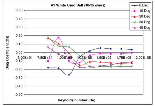
Figure 9.  $C_S$  variation with Re for used ball (10-15 overs)
