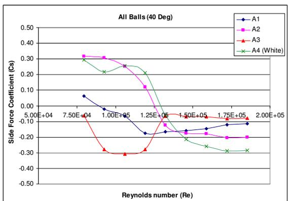
Figure 14.  $C_s$  variation with Re for all balls at 40° seam angle
