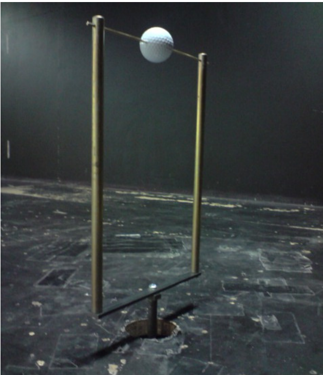
Figure 6. Mounting device on force sensor
