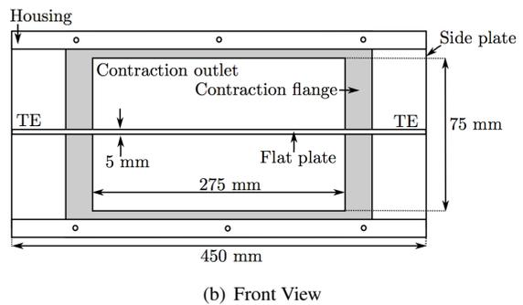
Figure 1: Test model without side walls.
