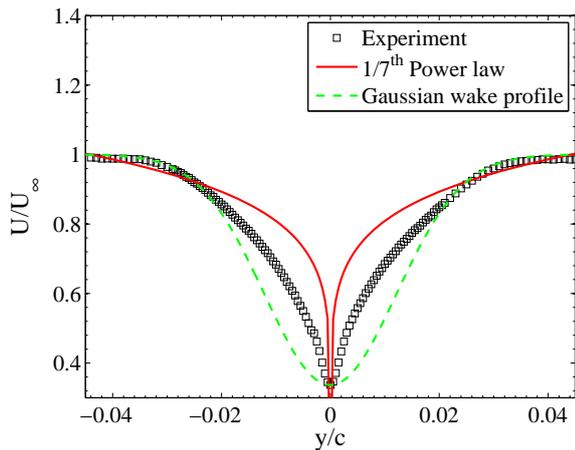
Figure 5: Mean velocity at the trailing edge.
