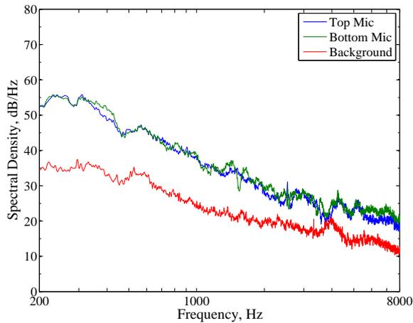
Figure 4: Noise measurements at  $U_\infty = 38$  m/s using no side walls and no boundary layer trips. The microphones were located 558 mm directly above and below the mid-span of the trailing edge. Wind socks were used on each microphone. Background measurements were taken using the top microphone.
