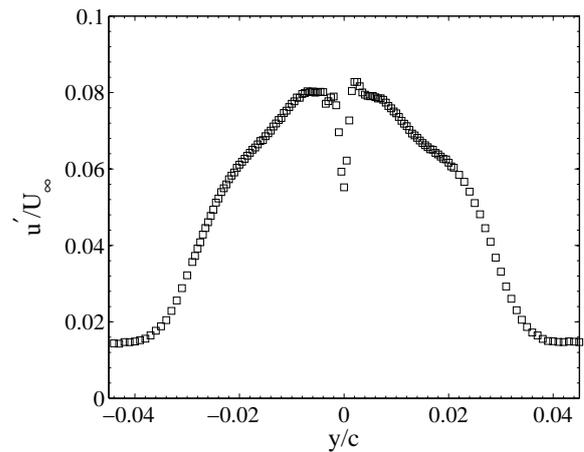
Figure 6: RMS velocity at the trailing edge.
