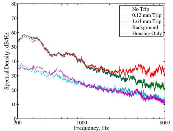
Figure 3: Single microphone noise measurements at  $U_\infty = 38$  m/s using no side walls and two boundary layer trips. No wind sock was used. The microphone was located 565 mm directly below the mid-span of the trailing edge.
