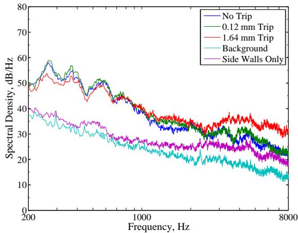
Figure 2: Single microphone noise measurement at  $U_\infty = 38$  m/s using side walls and two boundary layer trips. No wind sock was used on the microphone. The microphone was located 565 mm directly above the mid-span of the trailing edge.
