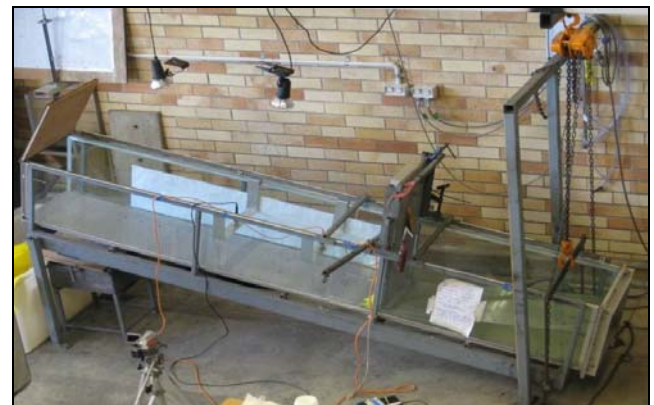
Figure 2. Dam break flume with an upward sloping bed and partially filled reservoir.
