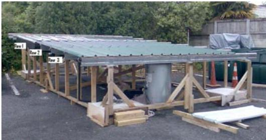
Figure 3: “Simulated” low slope roof, building integrated solar collector
