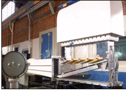
Figure 1. The large scale transonic planar cascade tunnel.
