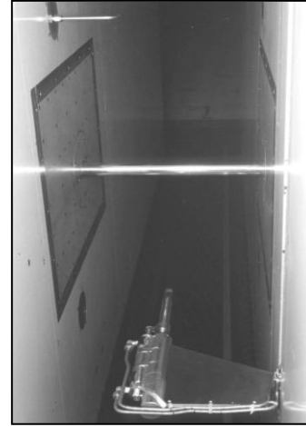
Figure 2. Circular cylinder mounted in the 1.5 m trisonic tunnel.
