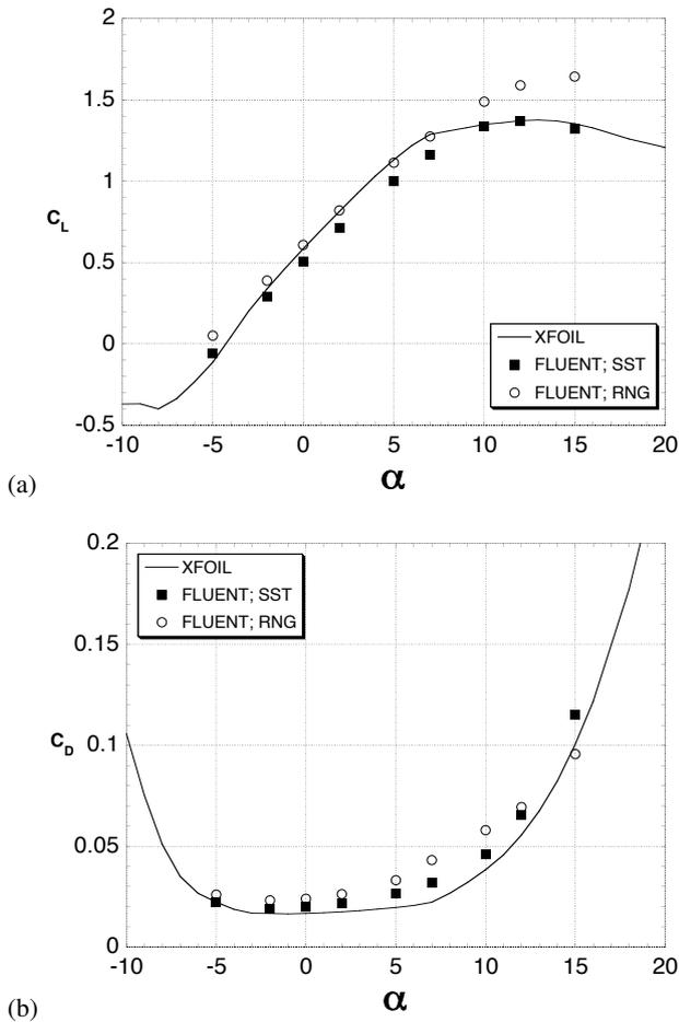
Figure 4:  $C_L$  and  $C_D$  calculated using the *XFOIL* and *Fluent* software.
