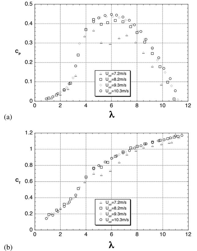
Figure 3: Experimental power and thrust coefficients. Reynolds number dependency tests.
