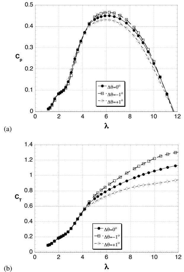
Figure 5: Performance predictions for three pitch angle settings using the BEM method.
