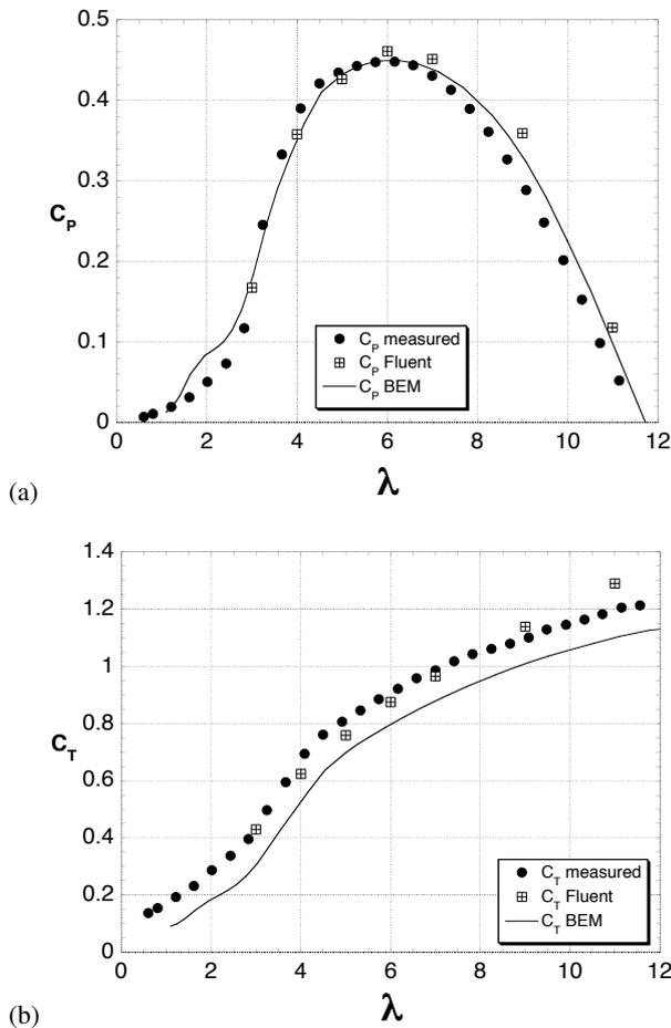
Figure 6: Comparisons of power and thrust coefficients from CFD and BEM with the measurements.
