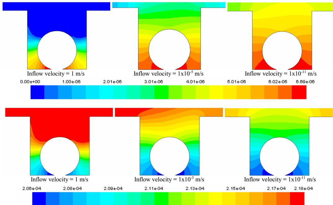
Figure 8: Lactate (top) and oxygen (bottom) concentration contour plots around the embryo for different inflow velocity.
