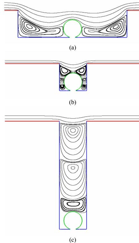
Figure 4: Streamline plots within the cavity for various cavity aspect ratios. (a)  $AR = 4.00$ ; (b)  $AR = 1.00$ ; (c)  $AR = 0.25$ . Note the streamfunction levels are not equi-spaced, but are chosen to highlight the recirculation regions.
