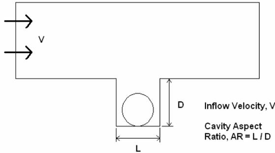
Figure 1: Schematic of the idealized cavity micro-bioreactor numerical model showing the two parameters to be studied.
