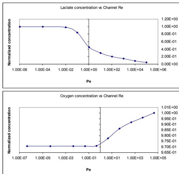
Figure 9: Lactate and oxygen concentration (normalized with respective highest concentration level) variation with Peclet number.
