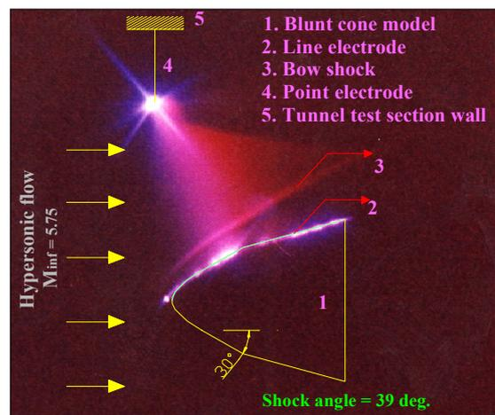
Figure 8: Shock structure around the blunt cone model.
