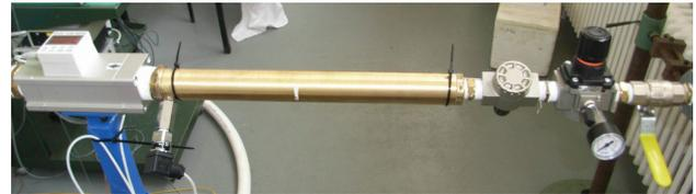
Figure 9. Coolant air metering components R-L: pressure regulator, needle valve, pressure transducer, flow-rate meter, thermocouple.
