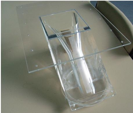
Figure 8. Cooling hole model machined from clear acrylic
