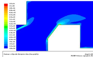
Fig. 15 Contour for Turbulent Eddy Dissipation Rate for 20% opening (k - ω model)
