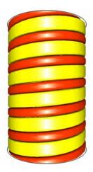
Fig.4. Laminar spirals in the system of infinite counter-rotating cylinders. Ri=110, Ro=0,  $\eta$ =0.8.
