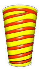
Fig.2. Laminar spirals in the system of conical cylinders. Ri=200,  $\alpha$ =16 degrees,  $\eta$ =0.84 at the top of the system,  $\Gamma$ =H/d=12.50. (H is the height of the fluid column, d the gap and  $\alpha$  the total (apex) opening angle of the conical cylinders). Isosurfaces show +/- radial velocity
