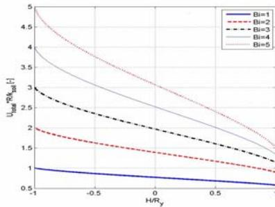
Figure 4. Shape factor as function of burial depth and Biot number.
