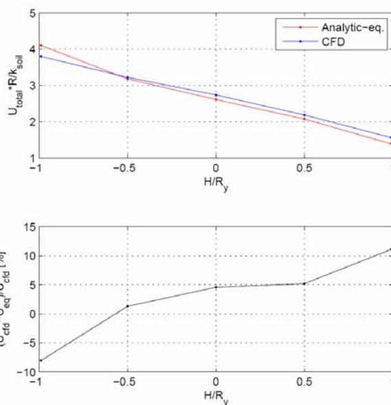
Figure 12. Comparison of the total heat transfer coefficient of the partially buried pipe.
