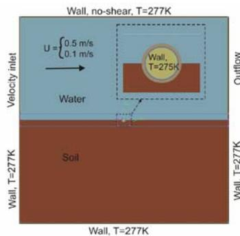
Figure 5. Geometry and boundary conditions for the CFD calculations
