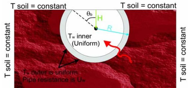
Figure 1. A partially buried pipe.
