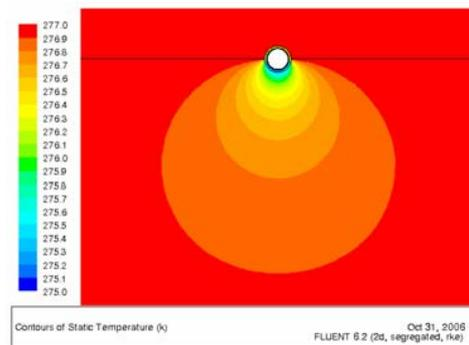
Figure 7. Temperature contours for a half-buried pipe
