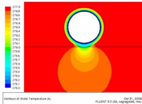
Figure 8. Temperature contours for a barely-buried pipe ( $H/R=-0.99$ )
