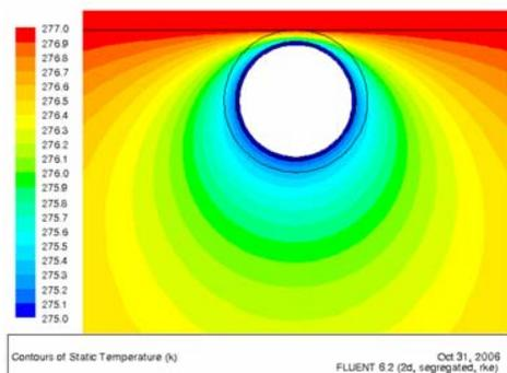
Figure 10. Temperature contours for a almost-buried pipe ( $H/R_y=+0.99$ )
