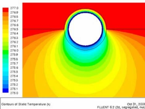
Figure 9. Temperature contours for a half-buried pipe ( $H/R=0$ )
