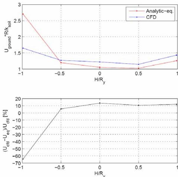
Figure 11. Comparison of the heat transfer coefficient of the buried part of the pipe circumference.
