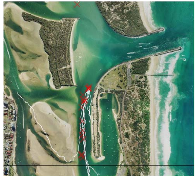
Figure 16. Drogue tracks (solid line is model simulation and red crosses are measured)
