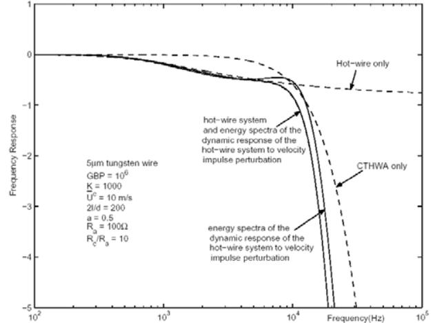
Figure 2 The normalized energy spectral densities from the dynamic response of the hot-wire system under different perturbations. Also shown are the frequency response of the hot-wire system as from Li (2004)
