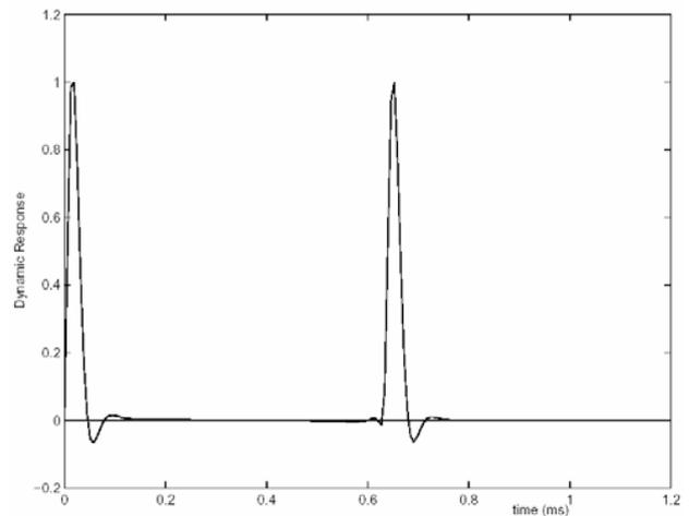
Figure 3 Dynamic response of the hot-wire system to a velocity impulse at the hot wire and that after applying the digital filter
