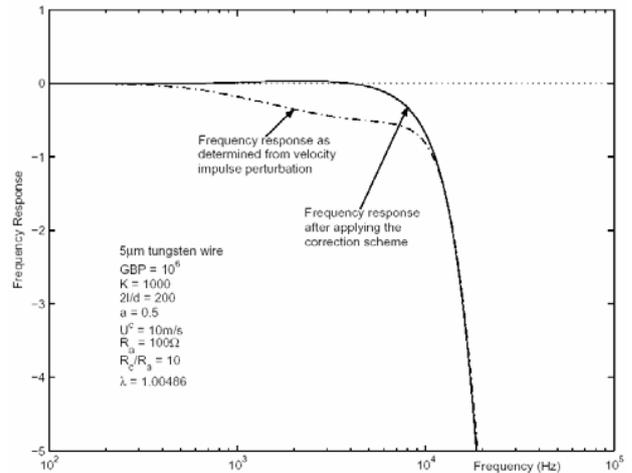
Figure 4 Frequency response of the hot-wire system under the velocity impulse, with and without applying the digital filter with  $\Delta U = 0.25U^c$ .
