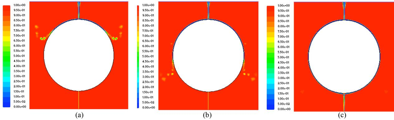
Figure 14. Falling liquid over the cylinder at different time where the air phase in red and water in blue, (a) the liquid film at the top of the cylinder; (b) at the centre of the cylinder; (c) the liquid film is complete around the cylinder.
