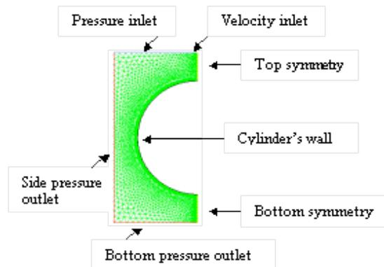
Figure 6. Half-domain numerical model with the boundary conditions.
