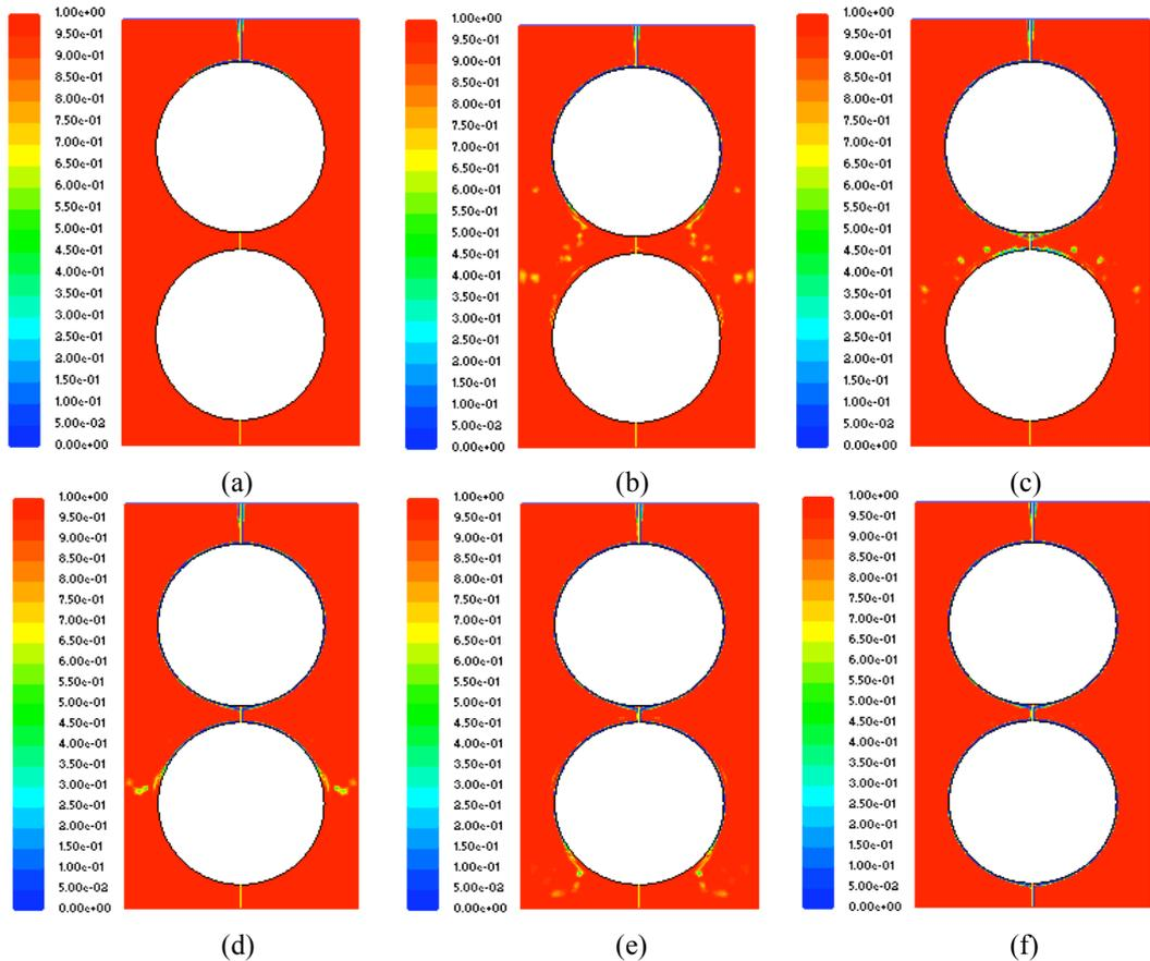
Figure 15. Falling film over two cylinders at different times (a) The liquid film over the top of the first cylinder; (b) at the bottom half of the first cylinder; (c) at the separation part between the two cylinders; (d) at the top half of the second cylinder; (e) at the bottom half of the second cylinder; (f) completion of the falling liquid film over the two cylinders
