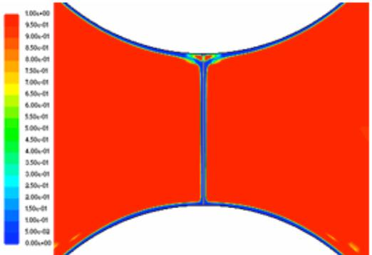
Figure 18. The separation is 0.03 m and the falling film is a sheet mode
