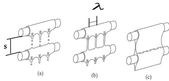
Figure 1. The idealized intertube of falling film modes; (a) droplet mode, (b) jet mode, (c) the sheet model. Mitrovic [5].
