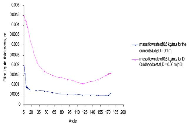
Figure 13. Comparison between the current study and Ouldhadad et al. [13].
