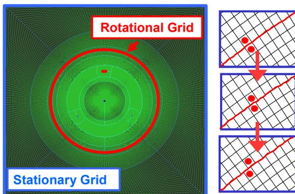
Figure 3 Computational mesh for numerical simulation for VAWT
