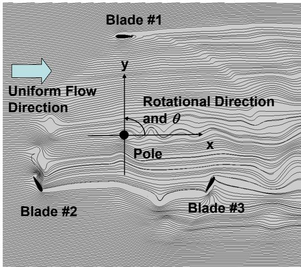
Figure 2 Schematic of Vertical Axis Wind Turbine and stream lines
