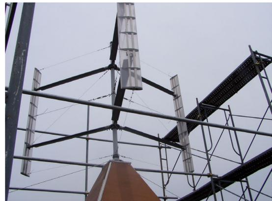
Figure 1 Vertical axis wind turbine with straight airfoils
