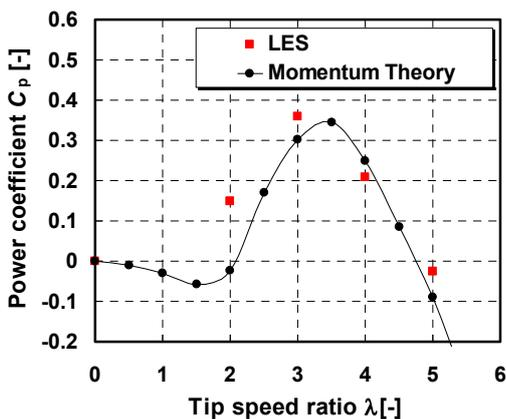
Figure 7 Power coefficient of VAWT
