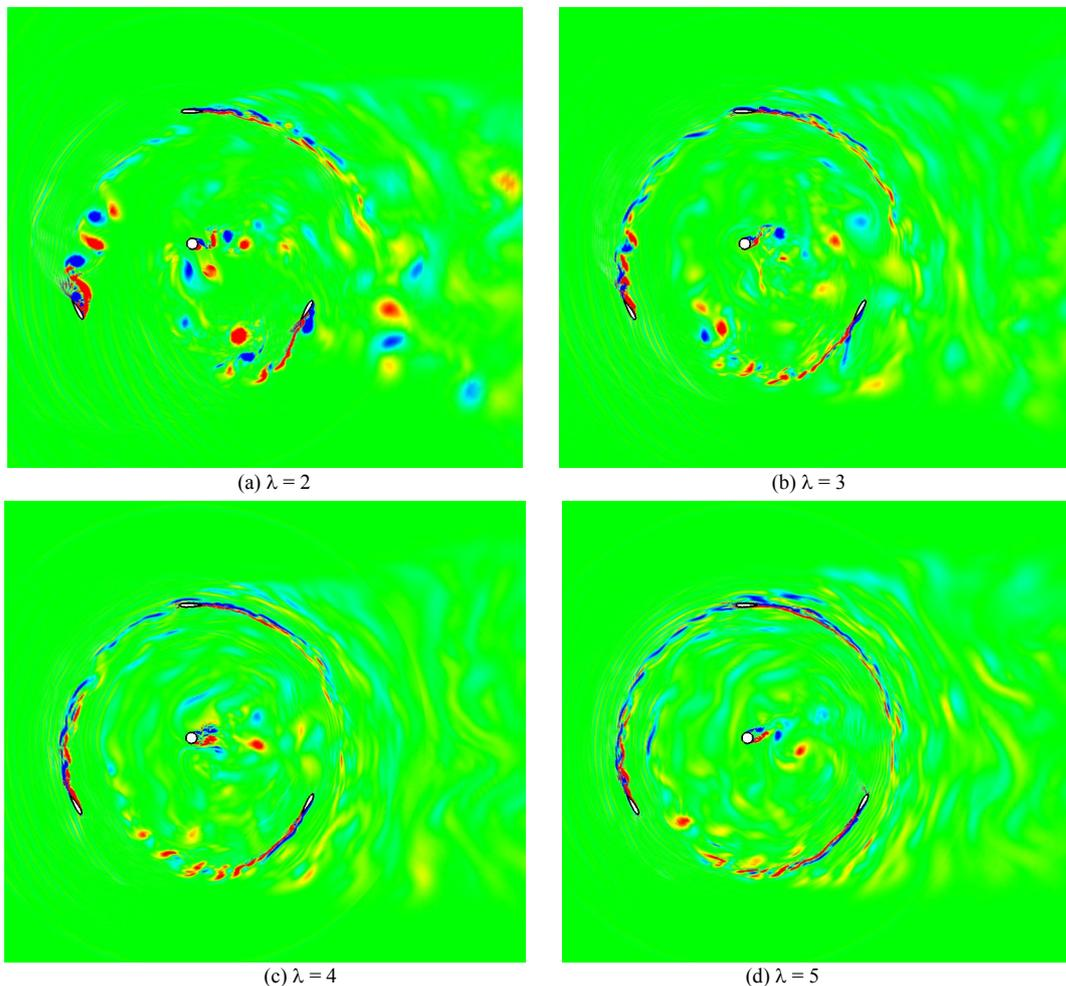
Figure 4 Vorticity distributions around a VAWT predicted by LES
