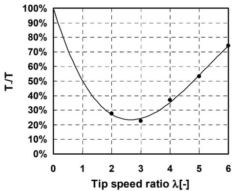
Figure 6 Ratio of negative torque period to rotational time of VAWT
