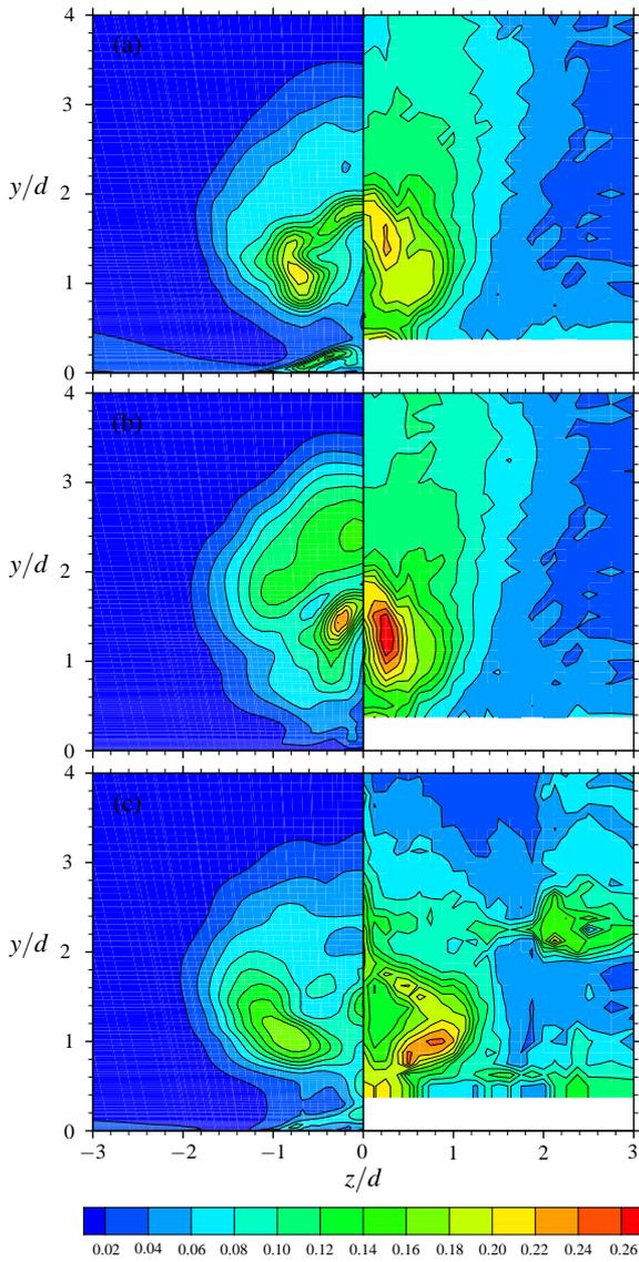
Figure 4: Dimensionless normal Reynolds stresses on the span-wise plane  $x/d = 3$ : FLUENT hybrid RANS–LES (left) and Santiago [4] experiment (right). (a)  $\langle u'^2 \rangle^{0.5}/U_\infty$ , (b)  $\langle v'^2 \rangle^{0.5}/U_\infty$ , (c)  $\langle w'^2 \rangle^{0.5}/U_\infty$ .
