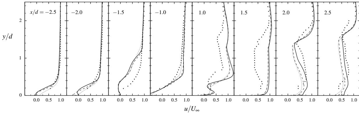
Figure 6: Dimensionless time-averaged stream-wise velocity profiles at various  $x/d$  stations on the stream-wise centreline plane: —, FLUENT hybrid RANS-LES (rke); ·····, RANS (rke); - - - , RANS (SST  $k-\omega$ ); •, Santiago[4] experiment.
