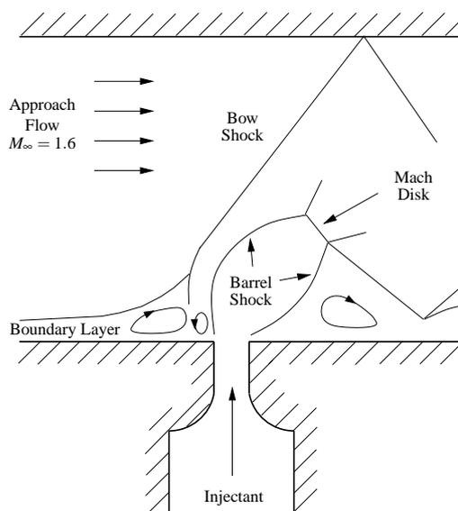
Figure 1: Schematic of injection into a supersonic cross-flow.
