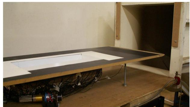
Figure 3 Cavity model with tunnel's side walls and roof removed.
