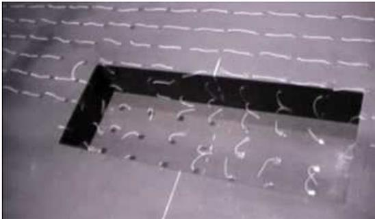
Figure 4 Photo of tuft flow visualisation experiments. Free stream flow from right to left.
