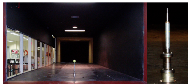
Figure 1: A front view of experimental set up in RMIT Industrial Wind tunnel with a motorised supporting device (right)
