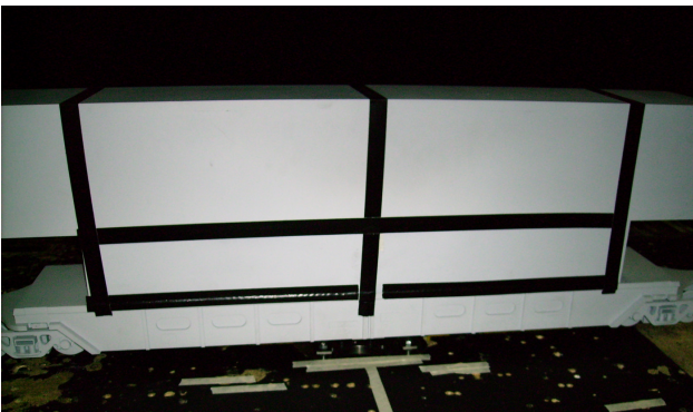
Figure 2a: Double Stacked Container Wagon at RMIT Wind Tunnel (SCT Logistics Configuration Type) – a Close View
