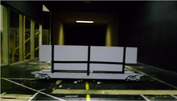
Figure 2: Double Stacked Container Wagon at RMIT Wind Tunnel (SCT Logistics Configuration Type)
