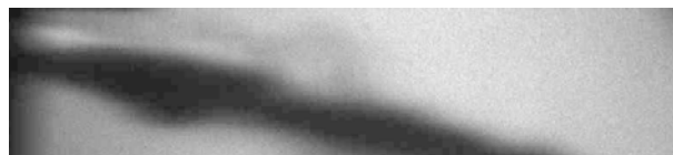
Figure 13. Schlieren image of a laboratory test 300 \mu s after diesel SOI and 100 \mu s after NG SOI. Diesel and NG injection pressures are 1,600bar and 160bar respectively.
