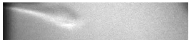
Figure 8. Schlieren image of the NG at 100 \mu s after SOI. The injection pressure is 160bar.
