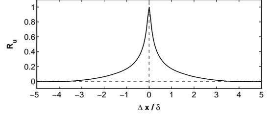
Figure 7: Autocorrelation curve from the fluctuating hot-wire  $u$  velocity signals. The spatial  $x$ -ordinate is obtained using Taylor's hypothesis and a convection velocity based on the local mean  $\bar{U} \approx 0.64U_{\infty}$ .
