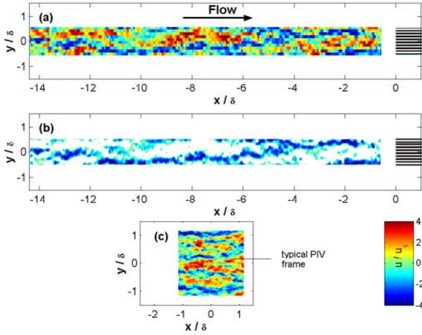
Figure 6: (a) Example signal section from ten sensor hot-wire rake at  $z/\delta = 0.14$ . Spatial view is reconstructed using local mean velocity ( $x = -U_{ct}$ ); (b) the negative momentum fluctuations only; (c) comparison with typical PIV frame.
