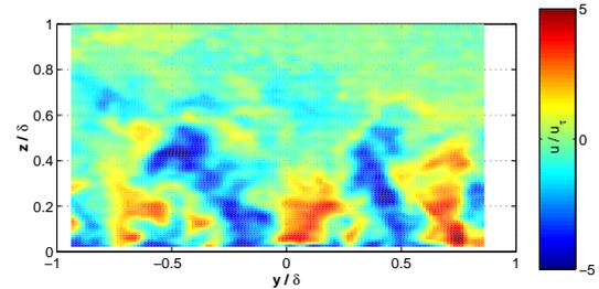
Figure 1: Example streamwise velocity field from  $45^\circ$  inclined plane. Color shading denotes velocity fluctuation.
