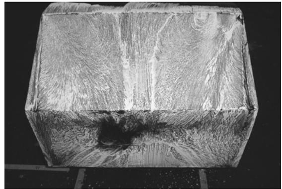
Figure 3. Rear end surface skin friction patterns.
