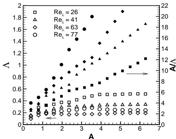
Figure 5: Integral length calculated from the autocorrelation function of vorticity over a range of spatial domains ( $A$ ). Also shown is the ratio of the spatial domain to integral length ( $L/\Lambda$ ). Results are shown for a range of  $Re_\lambda$ . Hollow symbols indicate  $\Lambda$ , filled symbols indicate  $A/\Lambda$ .
