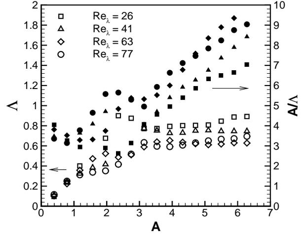
Figure 4: Integral length calculated from the longitudinal autocorrelation function over a range of spatial domains ( $A$ ). Also shown is the ratio of the spatial domain to integral length ( $A/\Lambda$ ). Results are shown for a range of  $Re_\lambda$ . Hollow symbols indicate  $\Lambda$ , filled symbols indicate  $A/\Lambda$ .
