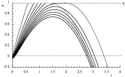
Figure 2: Selected Lagrangian trajectories,  $x_L(t)$ , under the overtopping flow (solid lines) when  $x_c = 1.0$ . Also plotted is the curve  $x = x_{ch}(t)$  across which the acceleration is discontinuous (dashed line).
