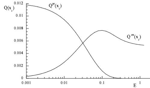
Figure 5: The net flux of sediment at the crest of the breakwater,  $Q(x_c)$ , as a function of  $E$  for  $q_e = u^2$  and  $x_c = 1.0$ . The internally mobilised,  $Q^{en}(x_c)$  and the presuspended components,  $Q^{pr}(x_c)$  are plotted separately.
