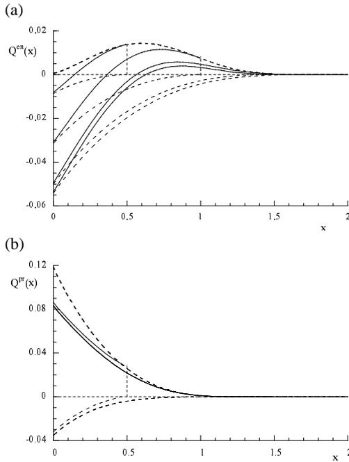
Figure 4: The net flux,  $Q(x)$ , across a breakwater with crest at  $x_c = 0.5, 1.0, 1.5$  and  $2.0$  for  $q_e = u^2$  and  $E = 0.1$  as a function of position: (a) Internally mobilised sediment,  $Q^{en}$ ; and (b) Pre-suspended sediment,  $Q^{pr}$ . The solid lines represent the net fluxes over the overtopping event; the dashed lines represent the contributions from the uprush and backwash components. (Note that in (b) the curves for  $x_c = 1.0, 1.5$  and  $2.0$  are indistinguishable.)
