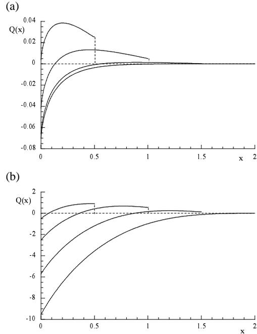
Figure 3: The net flux,  $Q(x)$ , across a breakwater with crest at  $x_c = 0.5, 1.0, 1.5$  and  $2.0$  for (a)  $q = u^3 h$ ; and (b)  $q = |u^3| u$  (Baillard model).
