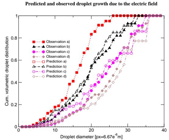
Figure 6: Comparison of the cumulative volumetric drop distribution obtained from the experimental observation and from the numerical analysis.
