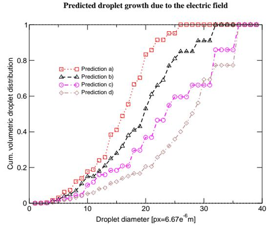
Figure 4: Cumulative volumetric drop distribution obtained from the numerical prediction of Fig. 3
