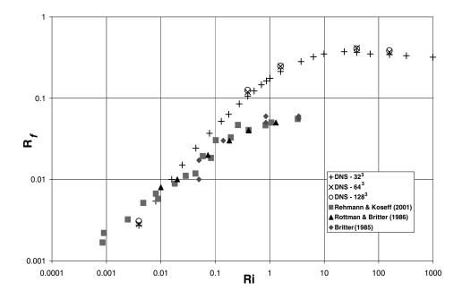
Figure 4: The mixing efficiency  $R_f$  plotted versus Ri for both experiments and DNS.  $\blacktriangle$ , experimental data from Rottman & Britter [7];  $\blacksquare$ , experimental data from Rehmann & Koseff [8];  $\blacklozenge$ , experimental data from Britter [1]; +, DNS at 32<sup>3</sup> resolution;  $\times$ , DNS at 64<sup>3</sup> resolution;  $\bigcirc$ , DNS at 128<sup>3</sup> resolutions. For the experiments,  $Pr \approx 7$  or 700, and for the DNS, Pr = 0.5.
