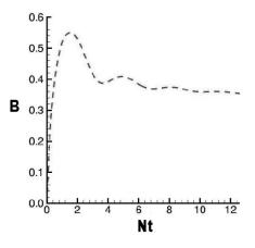
Figure 3: The evolution of the time-integrated buoyancy flux (non-dimensionalized with the initial turbulent kinetic energy) **B** as a function of time (non-dimensionalized by the buoyancy frequency *N*) computed by DNS for the case with Ri = 10 and Pr = 0.5.
