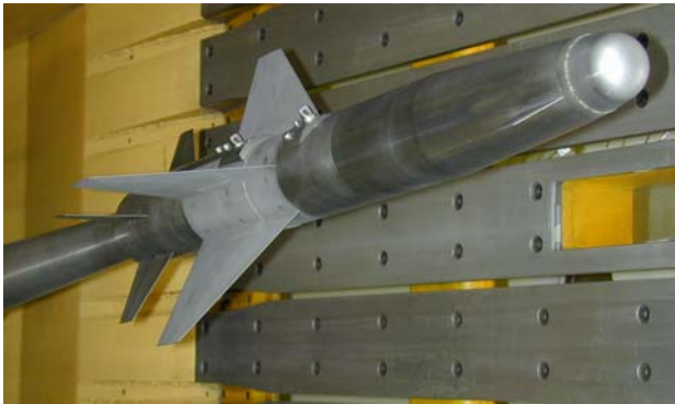
Figure 8. Store number 1 under test in the freestream
