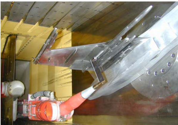
Figure 9. Store number 2 under test in the aircraft flowfield
