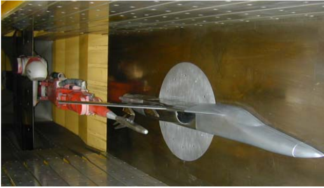
Figure 5. 6-DOF store model support with store (Number 1) under test in the flowfield of an aircraft half model
