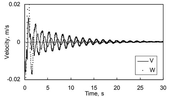
Figure 3. A time sequence for cross-stream velocities at a centreline point  $0.2D$  from the expansion ( $d=0.1$  m,  $U_i=10$  m/s,  $E=5$ ,  $L/D=1.0$ , no swirl).
