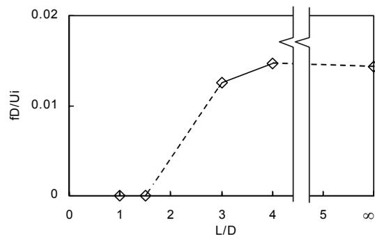
Figure 7. Variation of the precession frequency with pipe length ( $E=5$ , no swirl).
