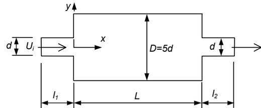
Figure 1. Schematic diagram of the geometry used in the simulation.
