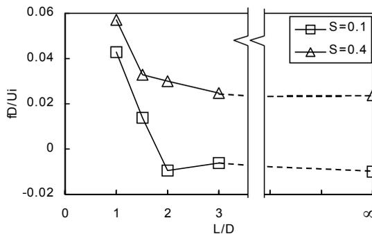
Figure 10. Variation of the precession frequency with the larger pipe length and inlet swirl number. (A negative value indicates that the precessing direction is opposite to the swirl.)
