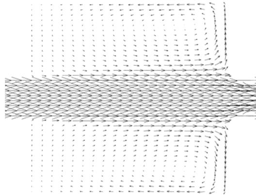
Figure 6. Vectors for steady flows showing a symmetric pattern ( $E=5$ ,  $L/D=1.5$ , no swirl).
