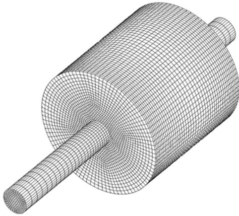
Figure 2. Typical grid used in the simulations ( $E=5$ ,  $L/D=1.0$ ).
