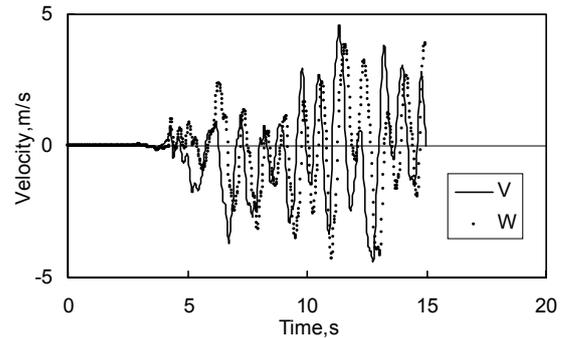
Figure 4. A time sequence for cross-stream velocities at a centreline point  $0.2D$  from the expansion ( $d=0.1$  m,  $E=5$ ,  $U_i=10$  m/s,  $L/D=1.0$ ,  $S=0.4$ ).
