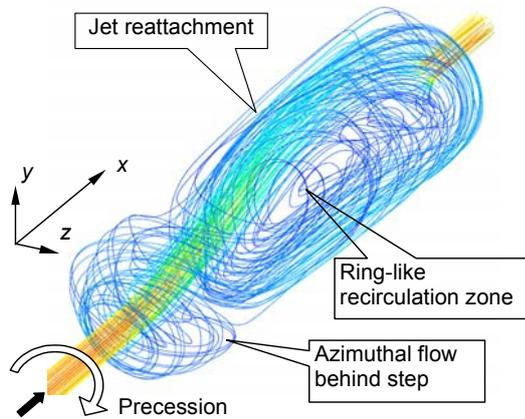
Figure 5. Instantaneous streaklines for precessing flow ( $E=5$ ,  $L/D=3$ , no swirl).
