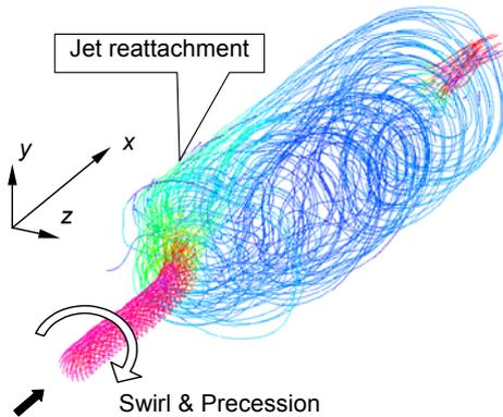
Figure 9. Instantaneous streaklines for precessing flow ( $E=5$ ,  $L/D=3$ ,  $S=0.4$ ).
