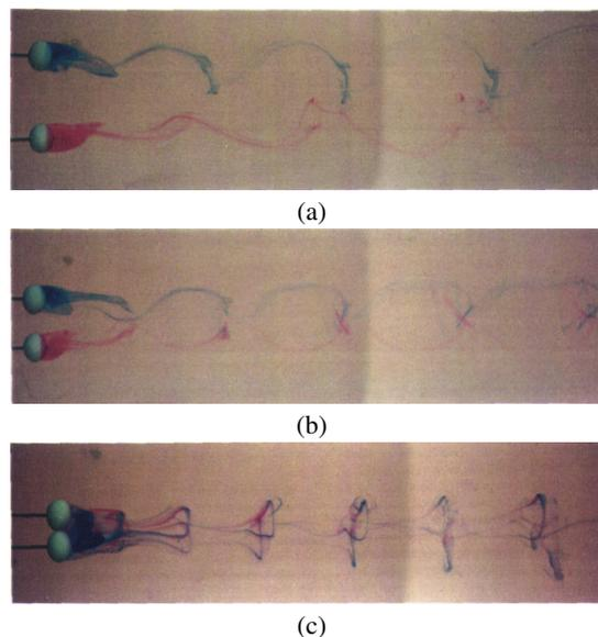
Figure 1: Experimental dye visualisations showing the change in the wake interaction as the separation is decreased. (a)  $S/d = 3$ , (b)  $S/d = 2$ , (c)  $S/d = 1$ , where  $S/d$  is the separation in terms of cylinder diameters.
