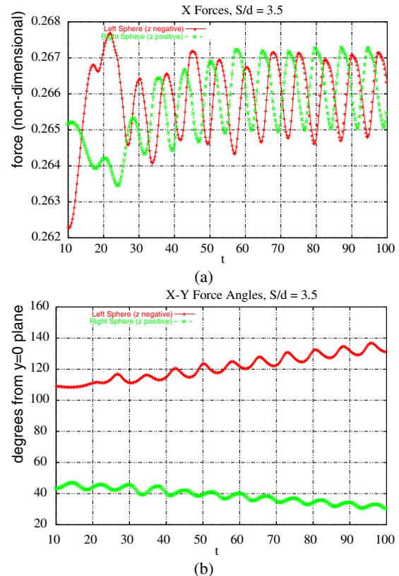
Figure 3: Forces on a two spheres at  $Re = 300$ ,  $S/d = 3.5$ . (a) Axial non-dimensional force. (b) Angle of non-axial forces on sphere.
