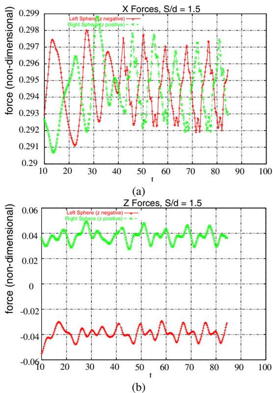
Figure 7: Forces on a two spheres at  $Re = 300$ ,  $S/d = 1.5$ . (a) Axial non-dimensional force. (b) Sideways forces on spheres.
