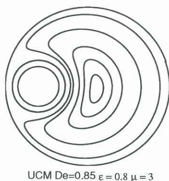
Figure 3: Streamlines for the UCM fluid with De = 0.85 , \epsilon = 0.8 , and \mu = 3 . The calculations were done on a mesh with 33 radial elements.
