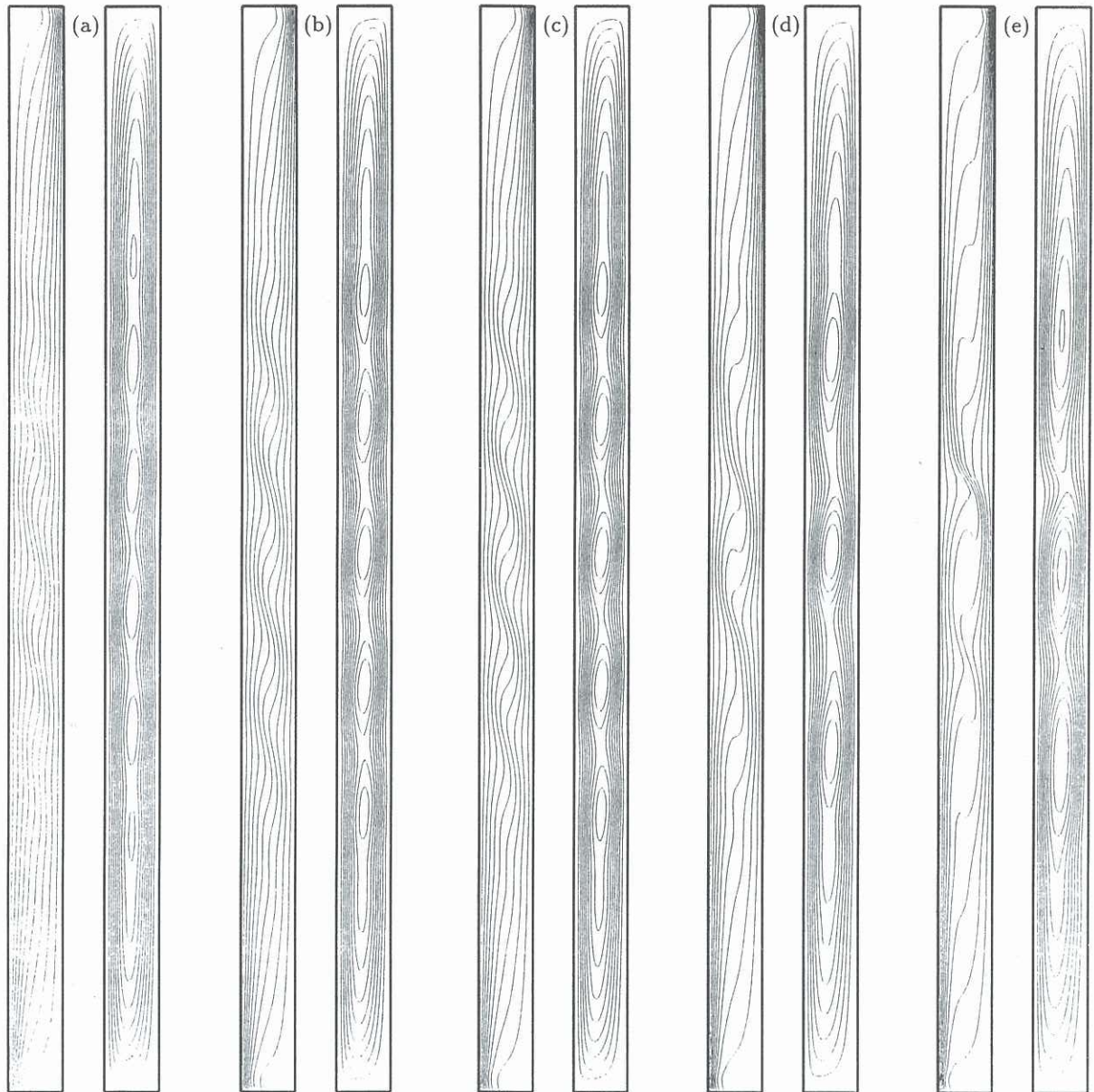
Figure 2: ASYMPTOTIC FLOW PATTERNS (TEMPERATURE AND STREAMFUNCTION) (a) Gr = 9,600 , 6 CELLS, (b) Gr = 11,000 , 5 CELLS, (c) Gr = 12,000 , 5 CELLS, (d) Gr = 25,000 , 3 CELLS AND (e) Gr = 50,000 3 CELLS
