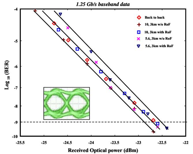
Fig. 6: Measured BER curves for baseband Ethernet data.
