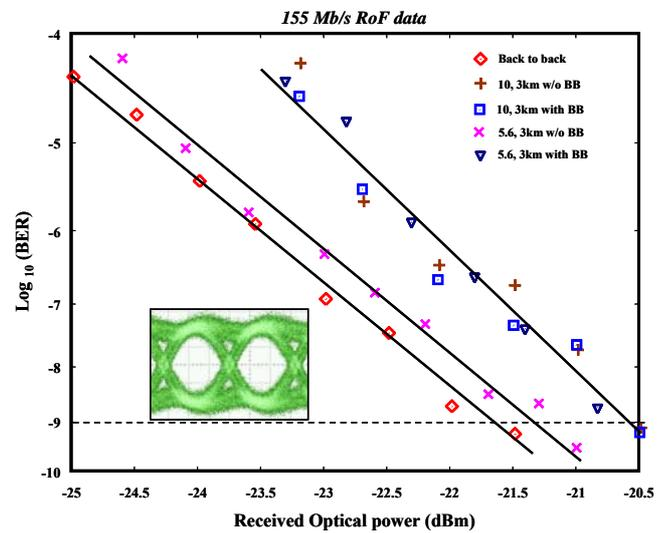
Fig. 7: Measured BER curves for RoF wireless data.
