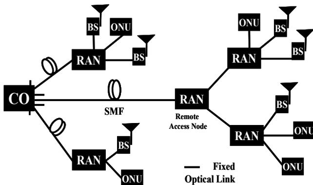
Fig. 1: Generic integrated optical network architecture.
