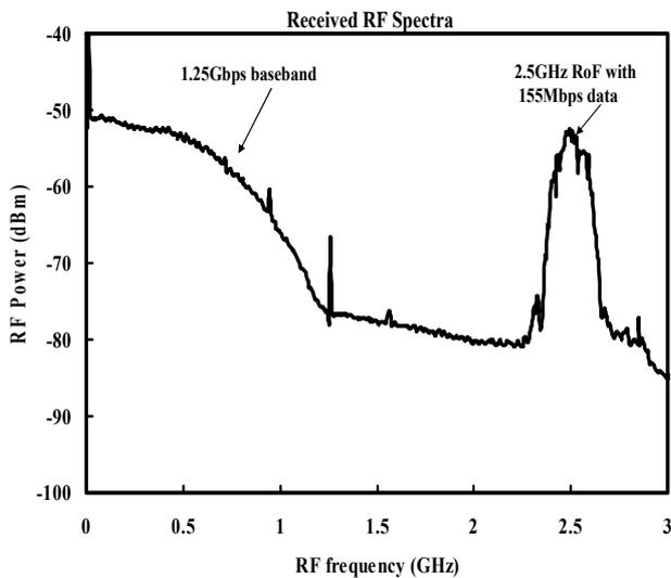
Fig. 5: Observed RF spectra showing the recovered RF signals at the PD and data recovery circuit.
