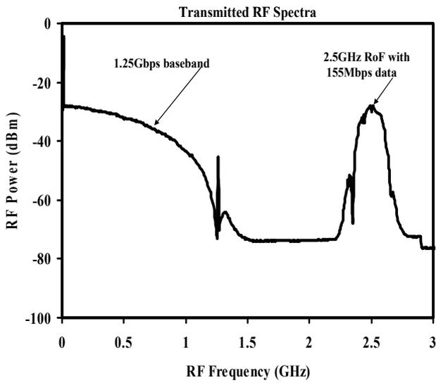
Fig. 4: Observed RF spectra showing the transmitted RF signals at the H-BS.
