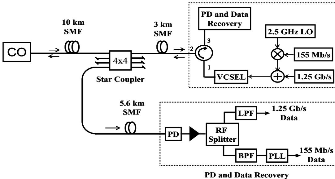
Fig. 3: Experimental setup for the demonstration of the proposed hybrid base station.
