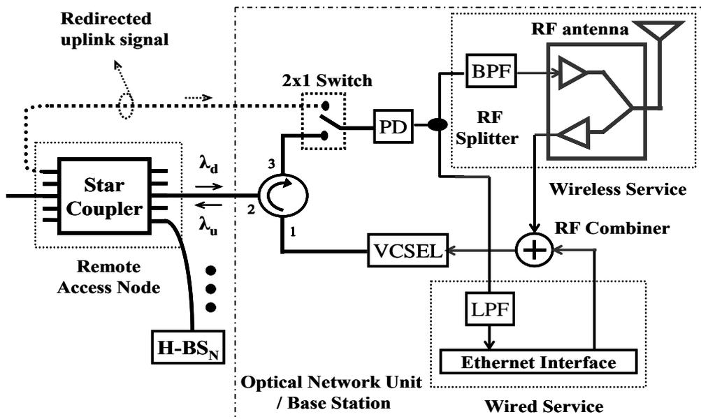
Fig. 2: Hybrid base station architecture providing simultaneous wireless and wireline services.
