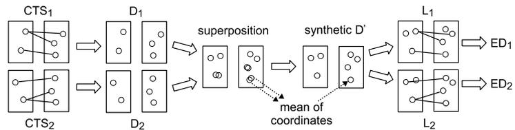
**Fig. 4.** An outline of the pairwise comparison procedure. Cells are represented with circles for convenience only. Cells need not to be round in videos.
