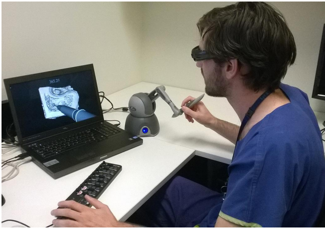
Figure 1: The University of Melbourne Virtual Reality Temporal Bone Surgery Simulator : it consists of a computer that runs a 3D model of a human temporal (ear) bone and a haptic device that provides tactile resistance to simulate drilling.
