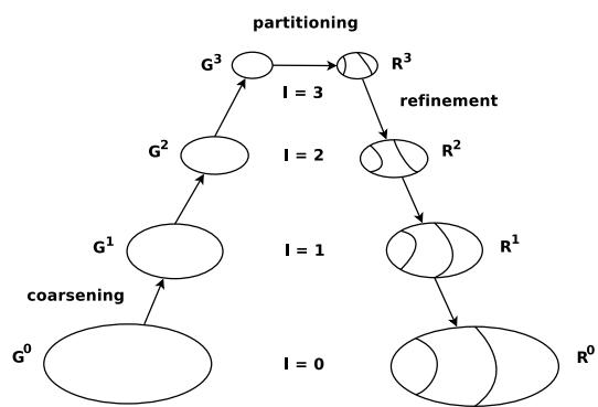
Figure 4: Illustration of the general multi-level graph partitioning process. The initial graph is labeled  $G^0$ , and the final partitions labeled  $R^0$ . There are four levels in this example ( $l = 0$  to  $3$ ).
