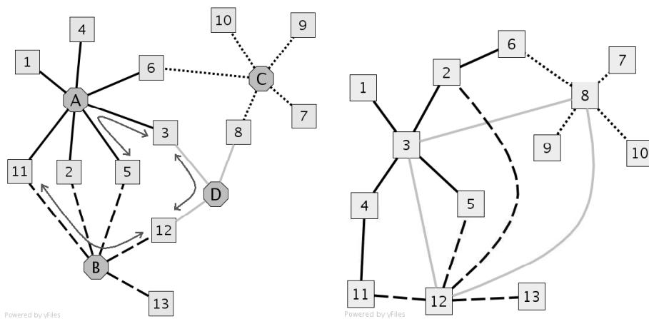
(a) Physical layer graph. The hexagons represent routers, and squares represent hosts. For ease of reference, all links connected to the same router have the same line style. Red, double headed arrowed lines are examples of the IP connections displayed in Figure 2b.
