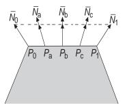
Normal vector interpolation used in Phong shading. What is the computational cost of Phong versus Gouraud?
