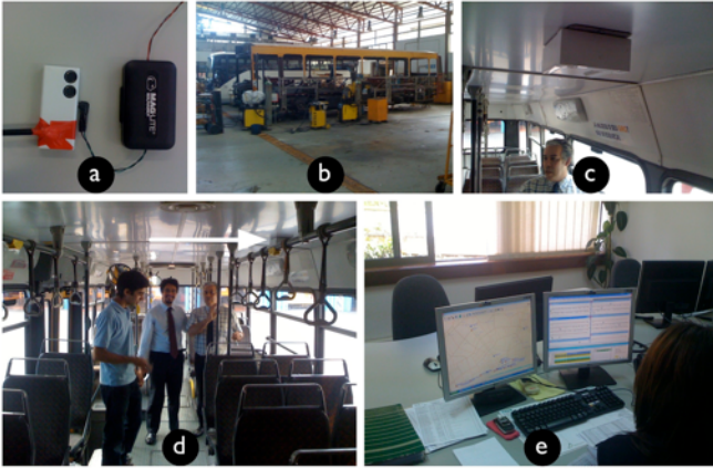
Figure 2. Installation of our system. a: The Gumstix computer (left), along with a 24 to 5 volt converter (right) used to power the Gumstix with the bus’ electric circuit. b: a bus being rewired. c: our final installation consisted of a protective plastic case attached to the roof of the cabin. d: the system (indicated with an arrow) is installed near the centre of the main cabin. e: the control centre where real-time data is gathered from the buses’ localisation systems and the whole operation is overseen.
