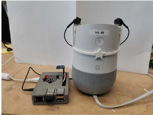
Figure 1: The Proactive Speaker Prototype.
