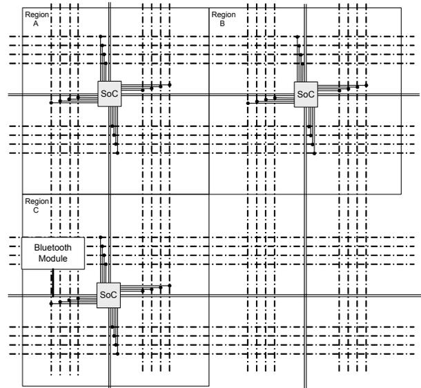
Figure 4. Textile electrical architecture. Regions A & B identical. Region C identical to A & B except additional Bluetooth™ module.
