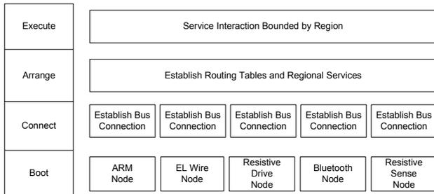
Figure 6. Execution environment layers
