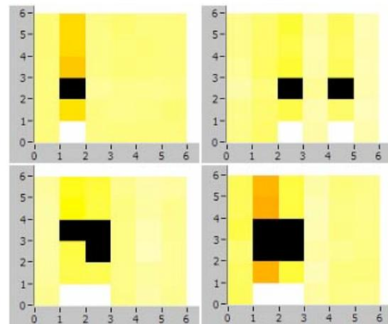
Figure 8. Crosshair isolation test. Intensity graph of resistive values over a 6x6 crosshair grid. Darker colors represent increased ADC values. Vertical is warp direction. Horizontal is weft direction. White through yellow represent crosshair noise floor. Labeled left to right, top to bottom: a,b,c,d.
