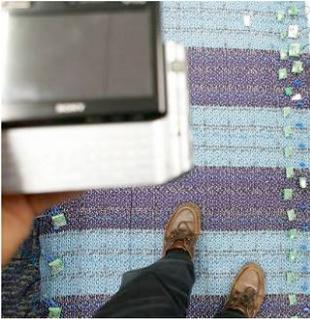
Figure 1. Ultra-Mobile PC associated through Bluetooth™ to electronic textile rug.
