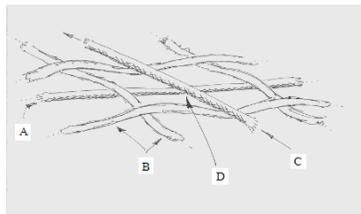
Figure 3. Resistive sensing in-fabric weave architecture. A & C steel wires. B wool fill & lift material. D sensing point.
