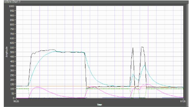
Figure 7. Single resistive crosshair test. Vertical axis: 10-bit ADC values. Horizontal axis: time. Darkest trace represents ball of foot press-hold-release(left) and press-release twice(right).
