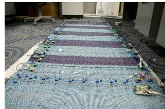
Figure 5. Final 3ft by 8ft textile prototype platform. Resistive sense(left edge). Resistive drive(top edge). Jumpered bus routers(bottom edge). CPU(bottom right). EL microcontrollers(right edge).
