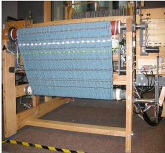
Figure 2. Initial rug on Virginia Tech's computer controlled loom.
