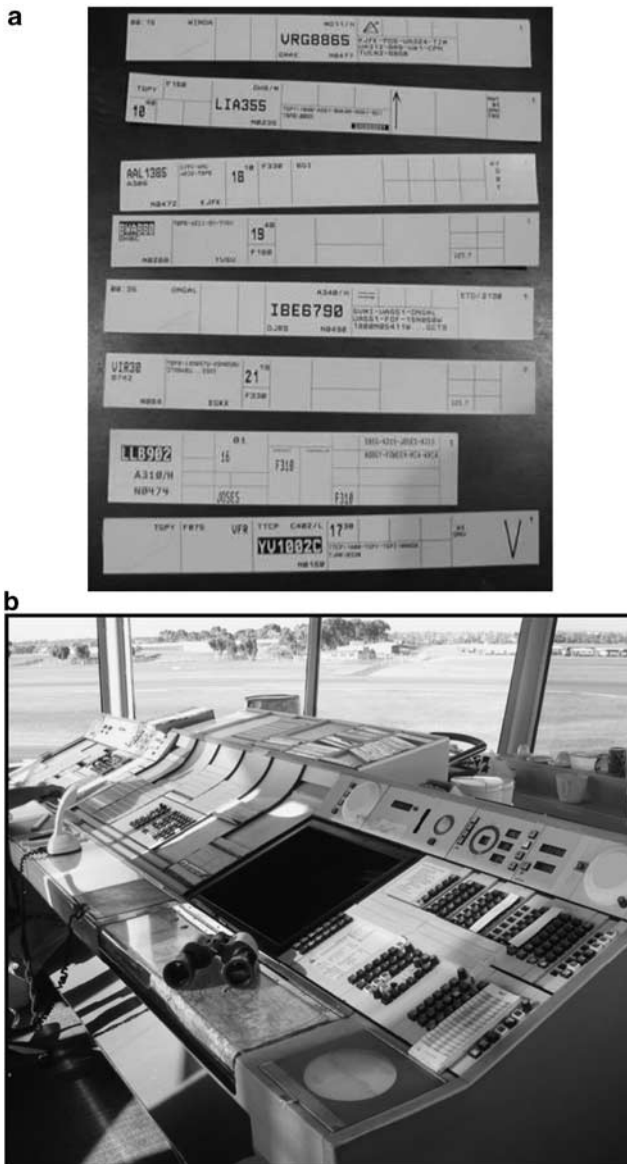
Figure 2 (a) Paper Flight Strips. discmd.com/atom/atom_functions/flight_strip_printing.htm . (b) Flight Strips in the Work Area. Essendon Airport, Victoria, Australia.
